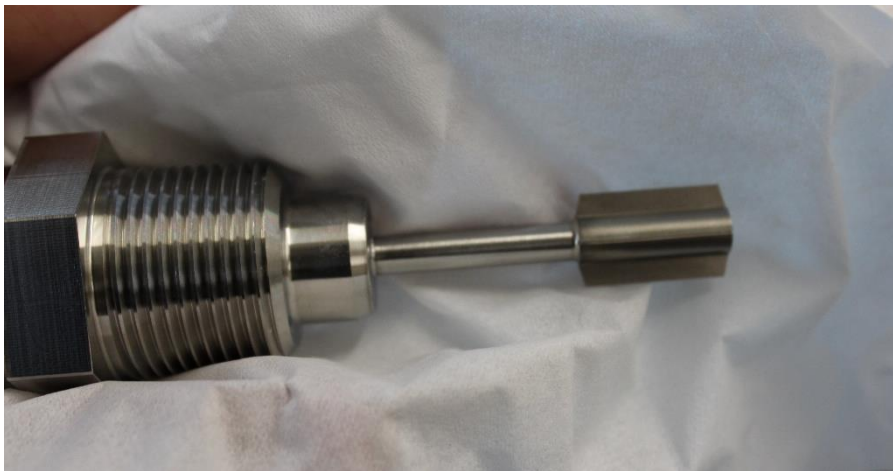
Cleaning the sensor with solvent-saturated cloth or paper
