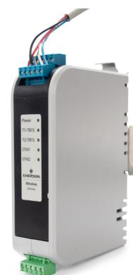
1: The WirelessHART adapter works with any gateway compliant with the WirelessHART (IEC 62591) standard; Rheonics can supply one if needed.
