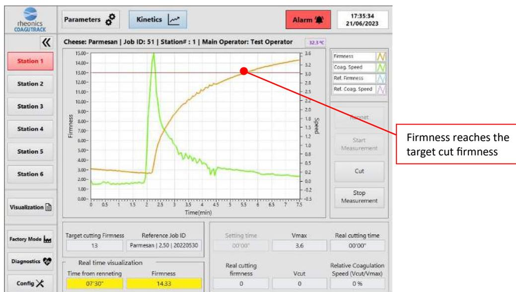
Figure 54 Cutting alarm active
