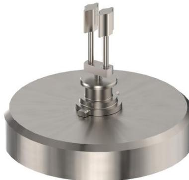
Figure 24: DV Sensor fixed on ORT Base
