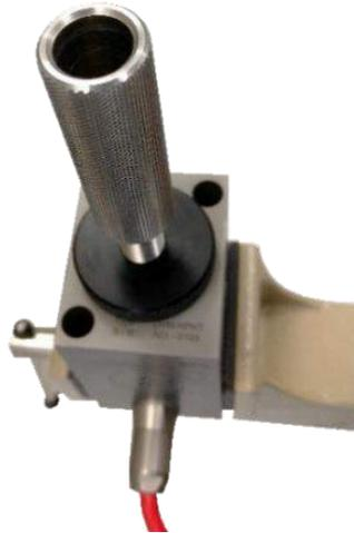
Figure 21: Threading the ERT-DVM into the DV sensor
