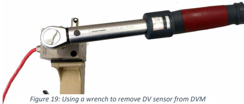
Figure 19: Using a wrench to remove DV sensor from DVM
