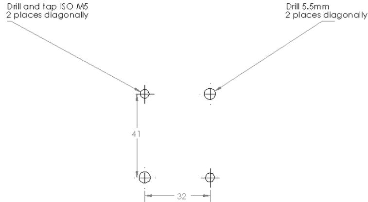
Figure 30: Mounting holes for DVM
