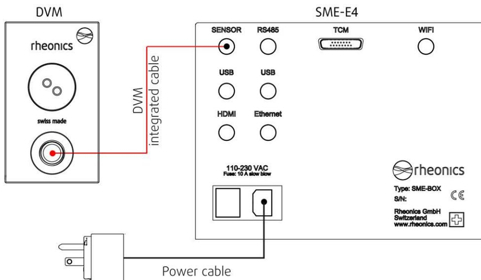
Figure 12: Rheonics sensor standard wiring for SME E4.
