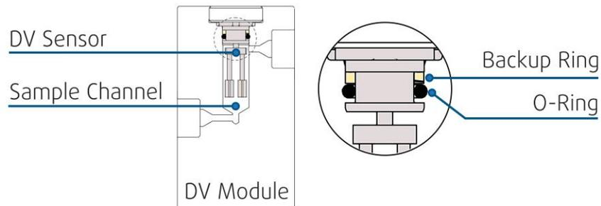
Figure 3: DV Sensor and sealing rings inside DVM
