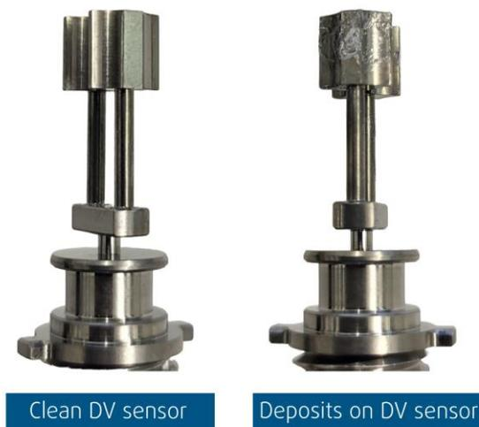
Figure 17: DV sensor clean and with deposits
