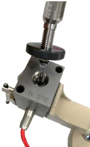
Figure 22: Removing the DV sensor from the DV module
