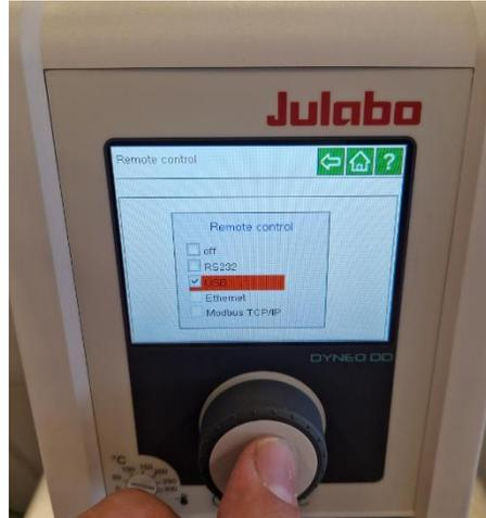
10. The display should say R-OFF, indicating the remote-control state. Set the temperature limit to the proper value. Turn the wheel in the bottom left to the maximum temperature that is safe for operation. This will depend on the fluid you fill in the bath. It is the responsibility of the operator to ensure the temperature limit is set correctly.
