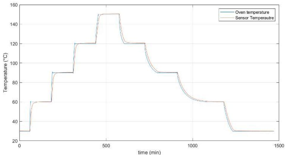
Accurate measurements require that the sensor temperature does not change over time, i.e. the sensor temperature is close to its thermal equilibrium which will be reached after a sufficiently long dwell time. Accurate measurements can be conducted after approx. 3600s. For high-accuracy measurements, Rheonics recommends a dwell time of 7200s.
