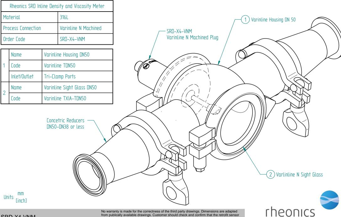
SRD-X4-VNM Housing DN50 Sight Glass - Reducers No warranty is made for the correctness of the third party drawings. Dimensions are adapted from publically available drawings. Customer should check and confirm that the retrofit sensor has the dimensions and flange specifications for a correct installation in their existing location.
