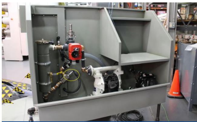
FIGURE 2. Installation of a symmetric resonator viscometer (SRV) using a flow adapter in an ink-delivery system (note the yellow oval)
