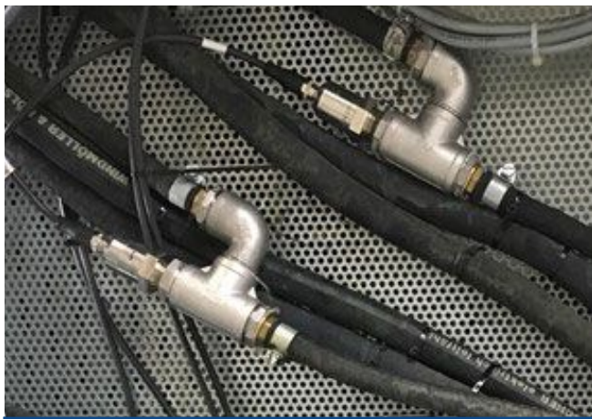
FIGURE 3. A symmetric resonator viscometer (SRV) installed on a press using a tee adapter
