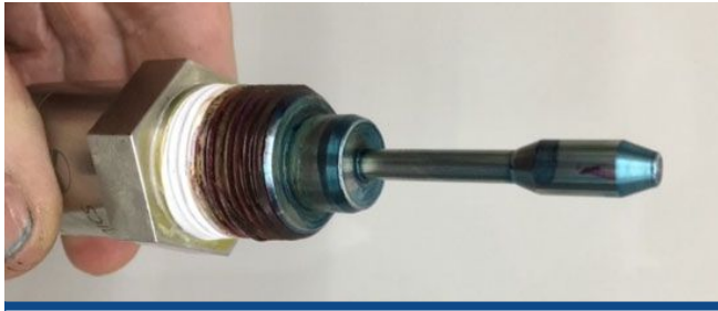
FIGURE 4. The SRV sensor after measurement in cyan ink
