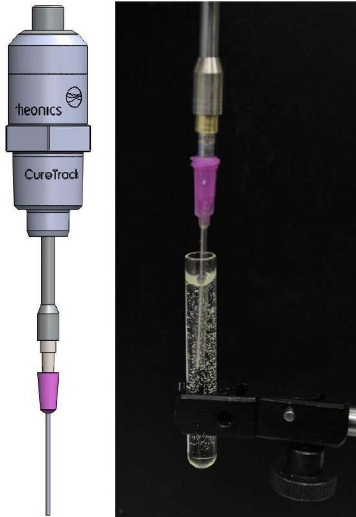
*Fig. 2: CureTrack instrument with closeup of sample tube and needle tip*
