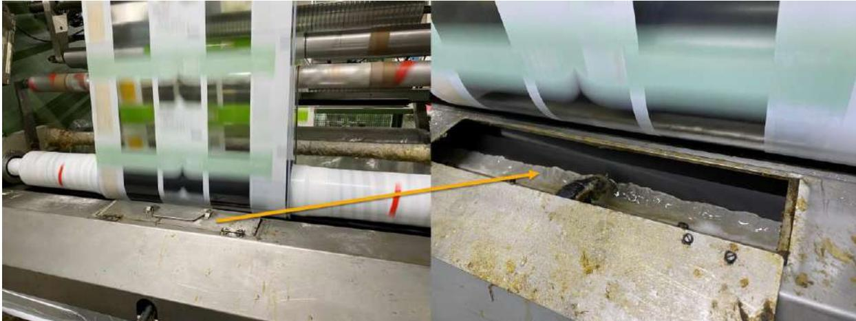
*Fig. 1: Adhesive reservoir in a high-speed laminating machine*
