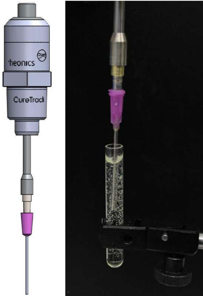
*Fig. 2: CureTrack instrument with closeup of sample tube and needle tip*
