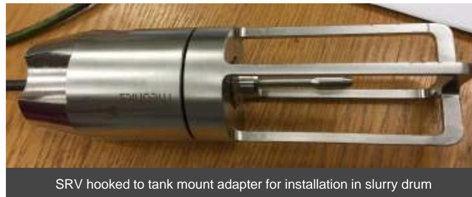
SRV hooked to tank mount adapter for installation in slurry drum
