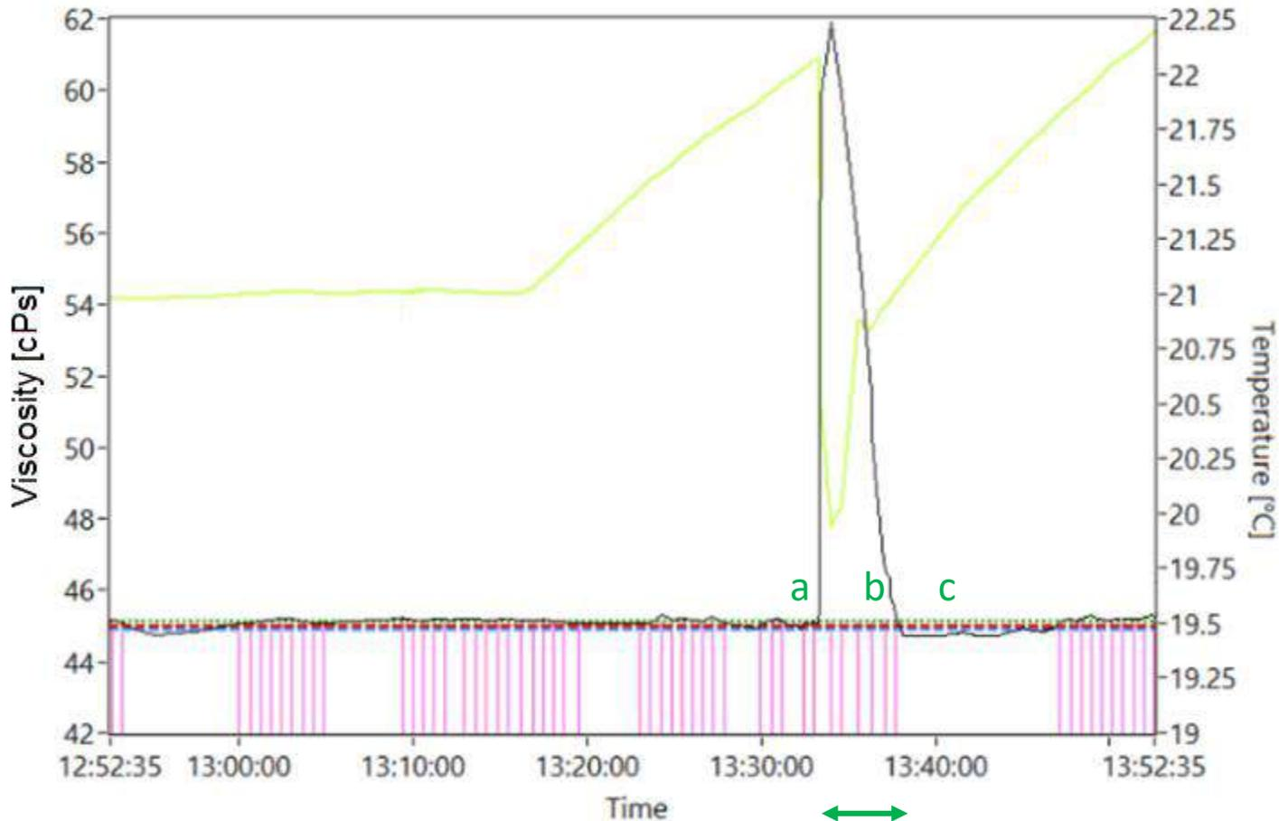
Rheonics integrated system brings viscosity to setpoint within 5 minutes
