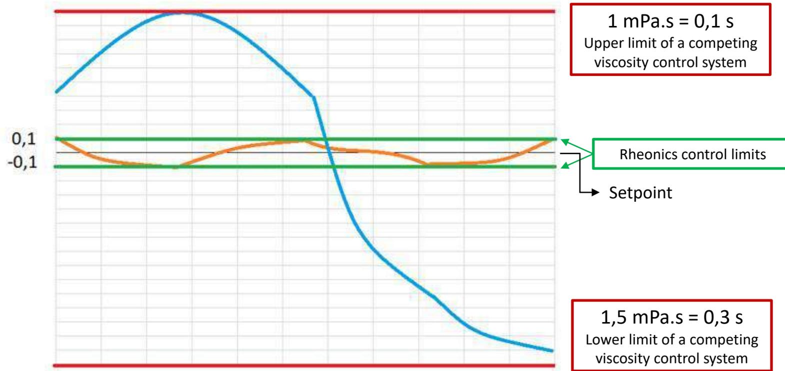
Exhibit – 1. Viscosity control accuracy, Rheonics SlurryTrack Vs.
