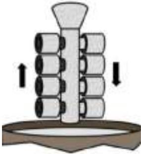
Viscosity is the single most important variable for shell quality and properties. SlurryTrack system helps maintain the highest quality, defects-free standards through tight and accurate viscosity control.
