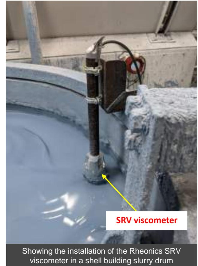
Showing the installation of the Rheonics SRV viscometer in a shell building slurry drum
