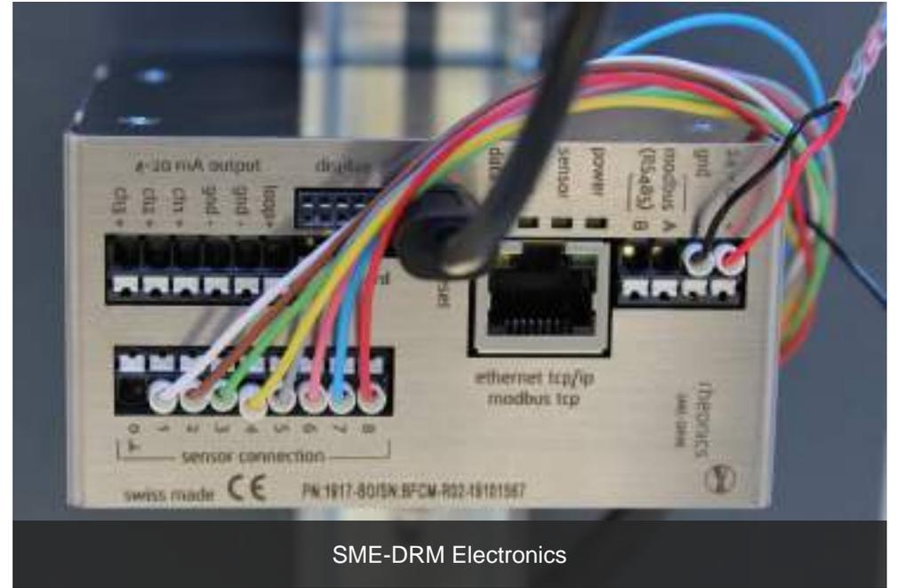
The SRV is connected to the SME-DRM electronics, which is connected to the customer PLC (using 4-20mA channels).
