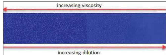
Figure 7: Color density variation with ink dilution and viscosity
