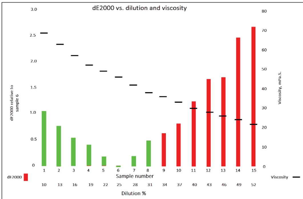
Figure 8: Color density as a function of ink dilution and density. Delta E 2000 values are referred to sample 6.
