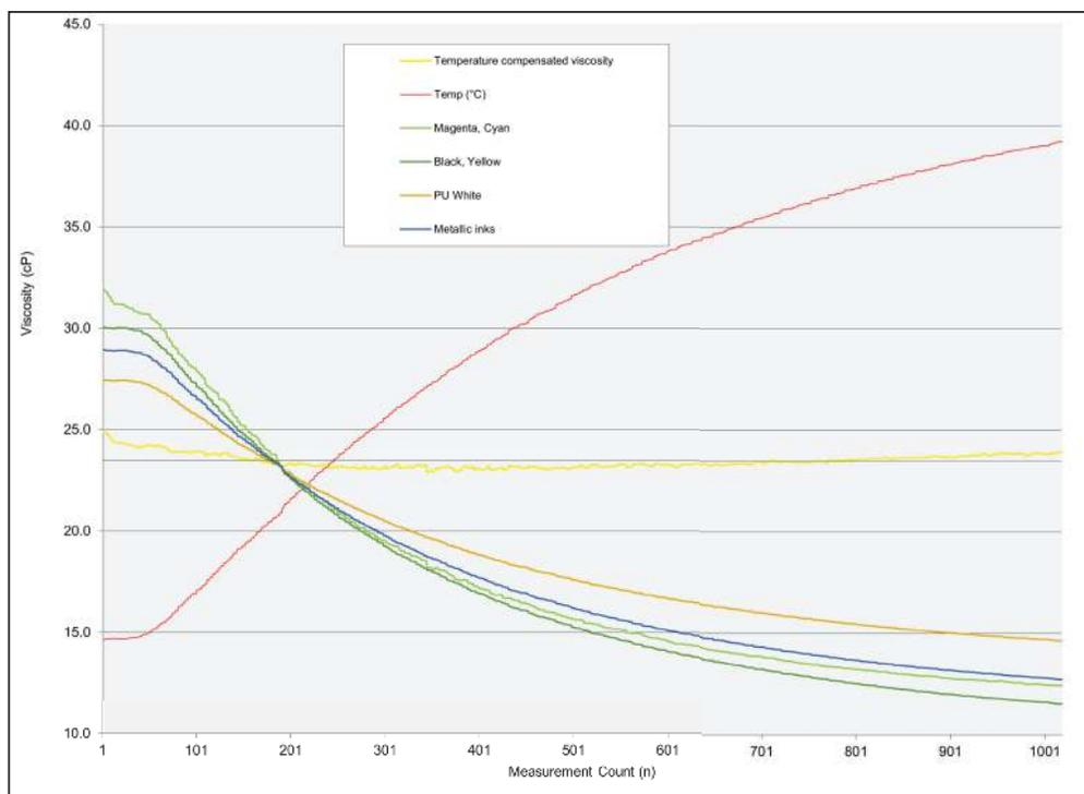
Figure 1: Temperature dependence of ink viscosity
