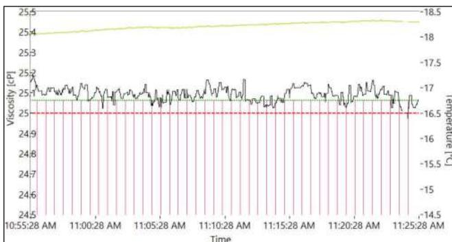
**Figure 5b:** Same plot as above, with expanded vertical scale. Temperature-compensated viscosity variation is less than 0.2 mPa.s.
