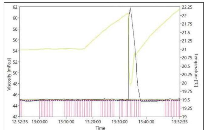
**Figure 6:** Response of the system to adding a large volume of cool ink to a system running at 21 degrees Celsius. Note the rapid recovery time of the temperature-compensated viscosity.
