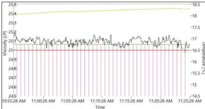
**Figure 5b:** Same plot as above, with expanded vertical scale. Temperature-compensated viscosity variation is less than 0.2 mPa.s.
