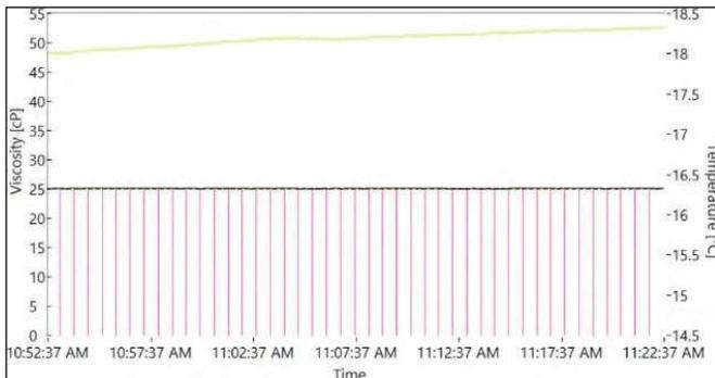
**Figure 5a:** Temperature-compensated viscosity (black, 25cP) and temperature (green, ~18 degrees Celsius) vs. time, coarse vertical scale
