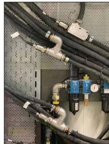
**Figure 4:** Four symmetric resonator viscometers installed on a press, using simple pipe tees as adapters
