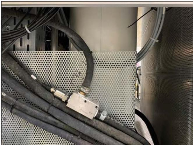
**Figure 2:** Sensor installed in ink line
