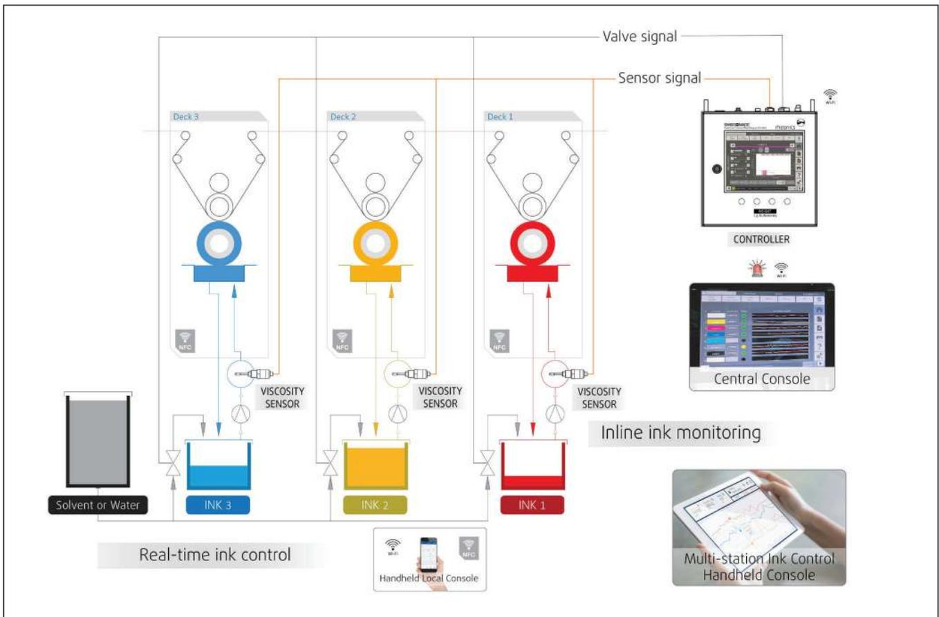
**Image 1:** Real-time ink control is achieved through inline ink monitoring facilitated by placement of viscosity sensors at each print deck. They connect and transmit data to central, multi-station and single-station handheld consoles.
