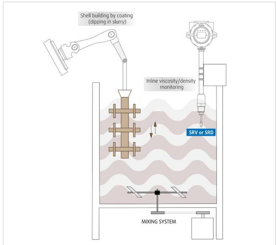
Figure 4: SRV/SRD in ceramic slurry mixing tanks during mixing and coating for shell building - Schematic with possible mount location of the sensor
