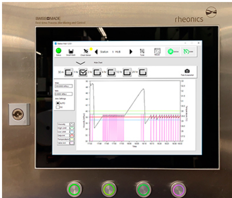
Combine inline viscosity sensors with Rheonics' Production Monitoring and Control System to obtain consistent viscosity of batter and product quality.
