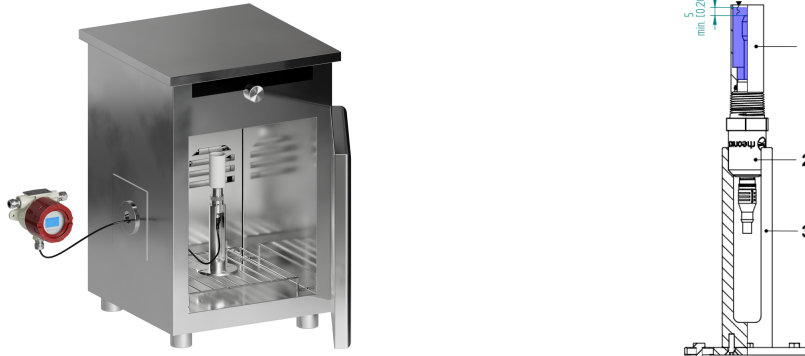
(a) Sensor probe placed in oven for thermal uniformity during calibration (b) Setup using Rheonics calibration stand and cylinder
