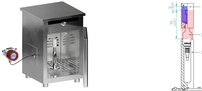
(a) Sensor probe placed in oven for thermal uniformity during calibration (b) Probe area required in thermal equilibrium for calibration
